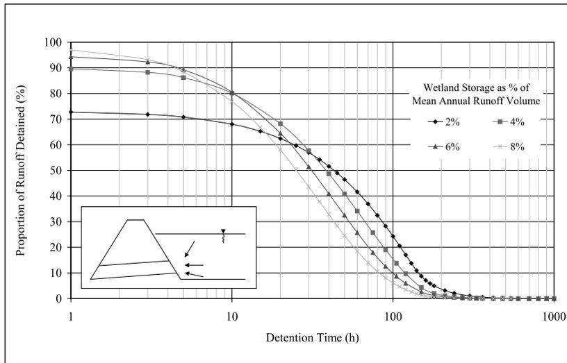
Figure 8: PRTD curves for a culvert outlet
