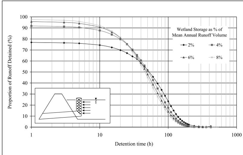
Figure 7: PRTD curves for a riser outlet
