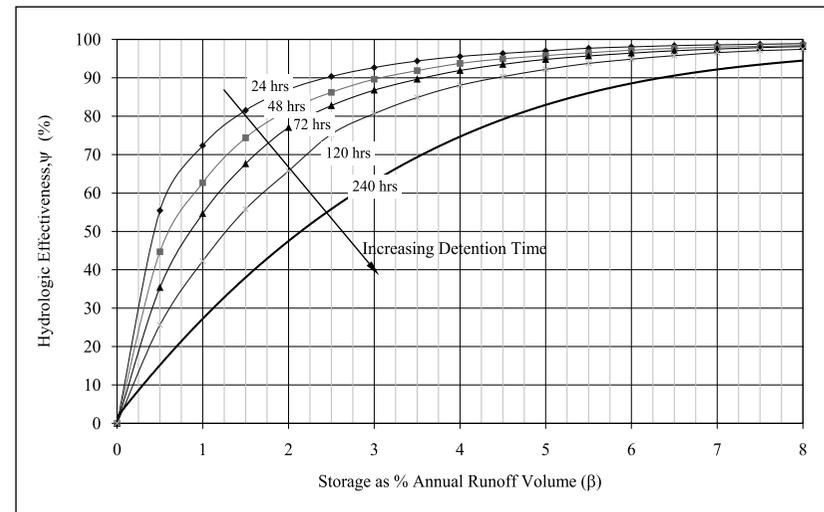
Figure 5: Hydrologic effectiveness curves for wetlands in Melbourne
