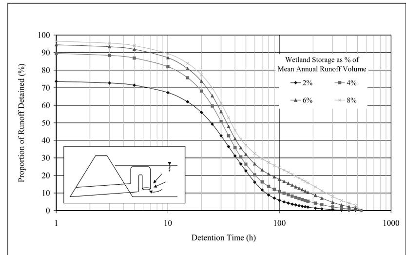
Figure 10: PRTD curves for a siphon outlet
