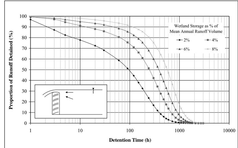
Figure 9: PRTD curves for a weir outlet
